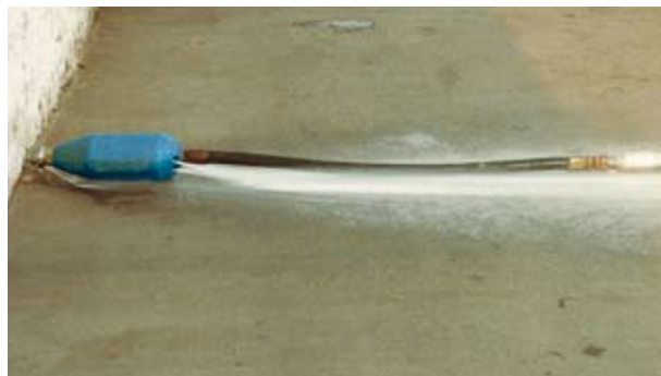
Reaction-force driven oscillating sewer cleaning Skip Jack
