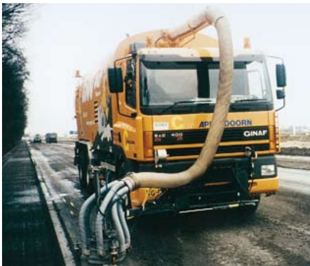
Municipal vehicle for sewer cleaning and emission-free stripping of white lines
