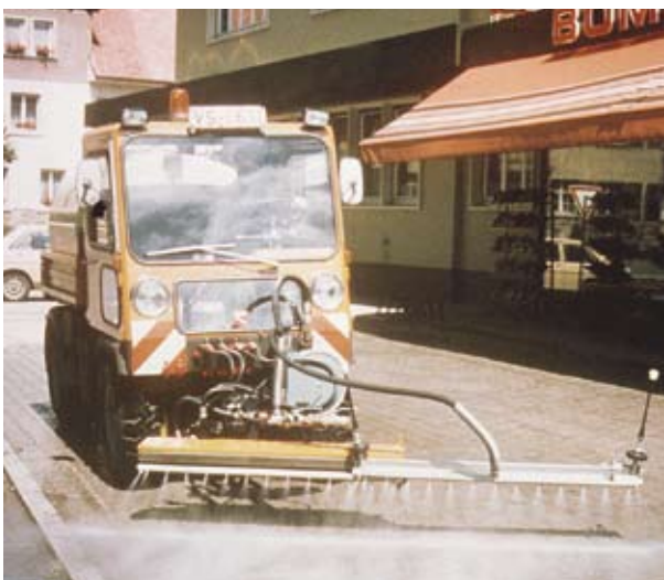
Road cleaning by high-pressure nozzle-beam and fan jets
