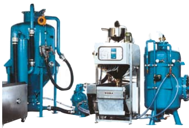
Modular treatment system for contaminated water
