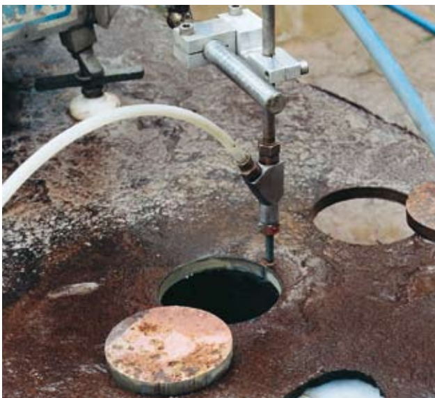
Cutting circular openings in steel plates
