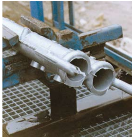
Removal of cast cores from suction pipes
