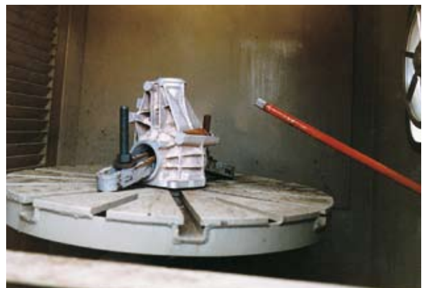
Cleaning of castings in a jetting cell
