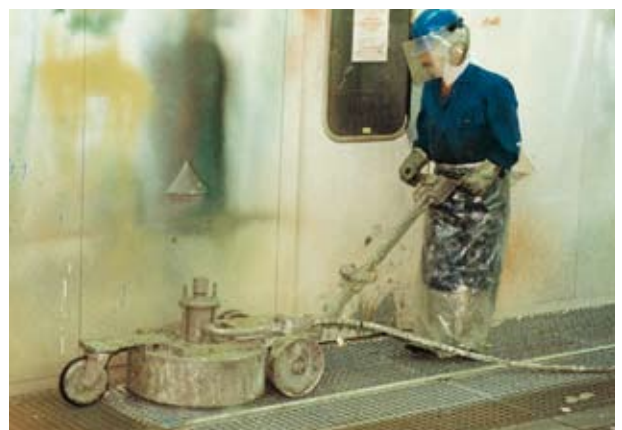
Cleaning of gridirons in enamelling cells
