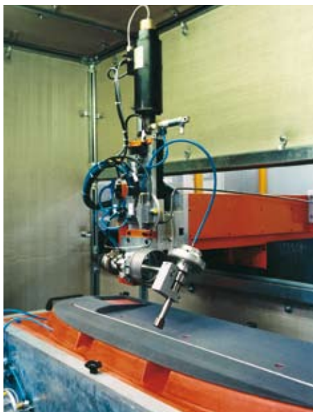
Deburring of oil ducts
