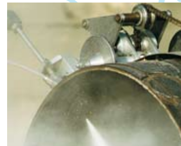
Pipe cutting with the high-precise abrasive water jet cutting system
