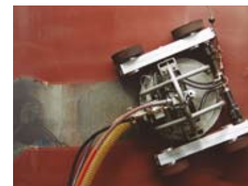
Lizard with remote control for emissions-free large-scale surface preparation
